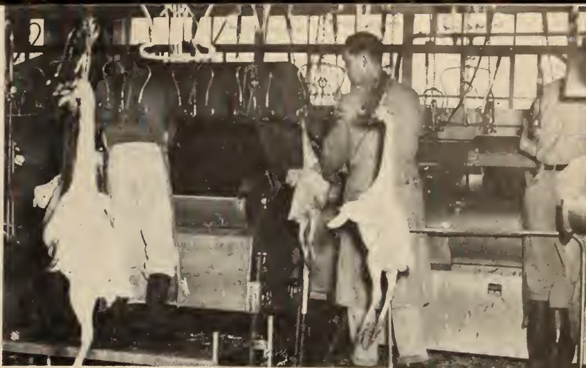
Flowline operation greatly speeds up the plucking of turkeys in this Portland, Ore., poultry plant. The birds are carried through tunnels and from machine to machine for different steps in the processing.
